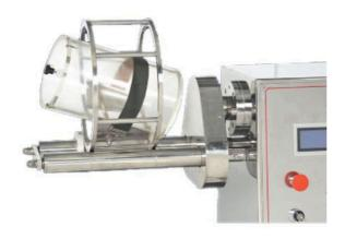
**DGN-2 Main Machine + Oscillating Granulator.** Oscillating Granulator adopts rocking and rotating granular solids to make granular solids pass the desired mesh belt, with its max productivity of 30 kg/h, wich depends on the materials and the meshes of two different sizes.
