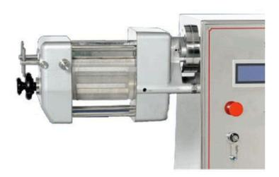
**DGN-2 Main Machine + Oscillating Sifter.** Vibrating screens. When rocking, it forces the granular solids to be screened by mesh, so you can choose the desired materials of mesh standard. There are screens of two sizes.
