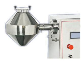
**DGN-2 Main Machine** + **Multi-Directional Movement Mixer.** Multi-Directional Movement Mixer. A ball barrel is bind symmetrically on the rotated frame, which is made of stainless steel, making the materials to be processed rotate as it and do three-dimensional motion, so as to rock-over and mix the materials.
